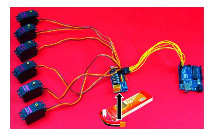
Always **connect GND of servo power supply** (one of the three black GND connectors beside screw terminal) to **Arduino GND**. Otherwise. It won't work.
