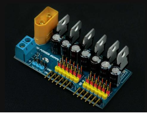
While working on a project that requires a bunch of servo motors (e.g.: a robotic arm), the first concern is to provide sufficient power to all of the motors. This module is useful to supply clean 5V to all of the servo motors of your project easily.
