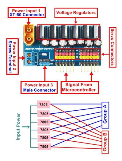
**Servo Connectors:** There are 12 standard servo connectors arranged in 2 groups.
